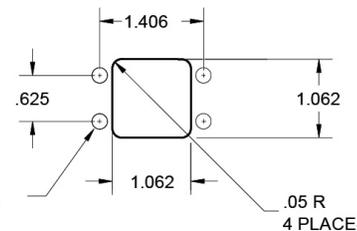
BOTTOM MOUNT-CLEARANCE HOLE FOR .192 SCREW
